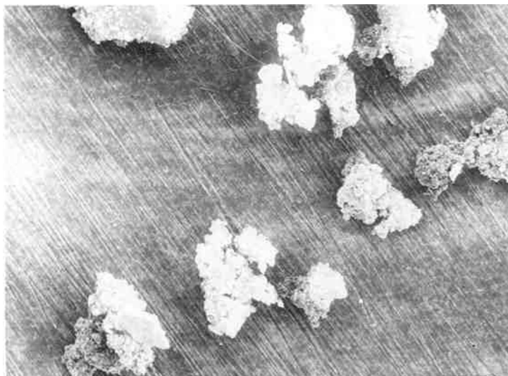
Fig. 3. Scanning electron micrograph of powdered rubber rejects.
